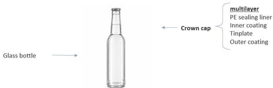
Figure 4: Glass bottle with crown cap
